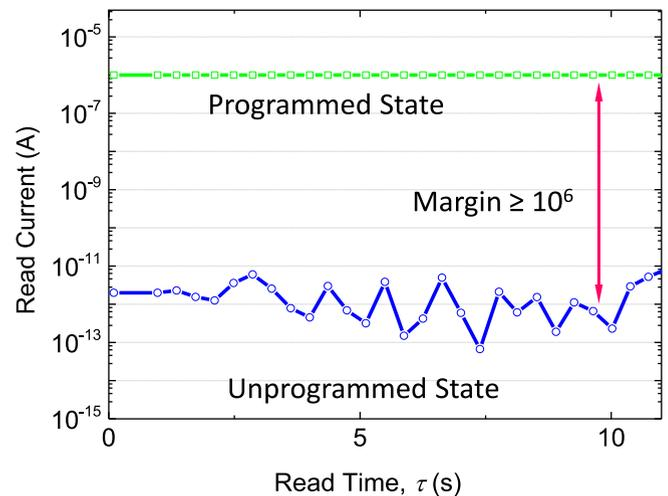
**FIGURE 15.** Read sweep before/after programming cycle in Fig. 14(b) and (c) showing large read margin between the programmed/unprogrammed memory cell, exhibiting a read margin of over six orders of magnitude.
