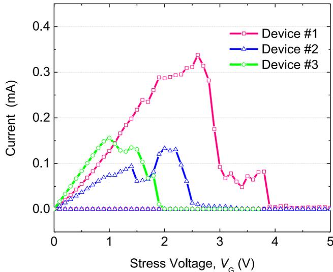
**FIGURE 7.** Programmed NEMS antifuses breakdown process under high currents.
