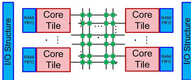
**FIGURE 1. Schematic architecture of Microsemi Axcelerator antifuse FPGA. The major components include core tiles containing the logic blocks, RAMs, and data buffering for storage and I/O structure for inputs and outputs. Green squares are antifuses. FIFO stands for first-in and first-out.**
