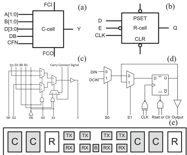
**FIGURE 11.** Schematic of the basic logic blocks in Axcelerator antifuse FPGA. (a) C-cell. (b) R-cell. (c) and (d) Gate-level schematics of C-cell and R-cell with input and output signals, respectively. (e) SuperCluster block comprised of C-cells, R-cells, and transmit and receive routing buffers, in Axcelerator antifuse FPGA.
