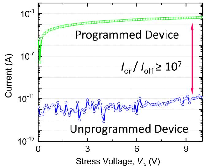
**FIGURE 6.** Stress voltage sweep on programmed and unprogrammed NEMS antifuse showing a large on/off ratio between programmed and unprogrammed interconnect devices.
