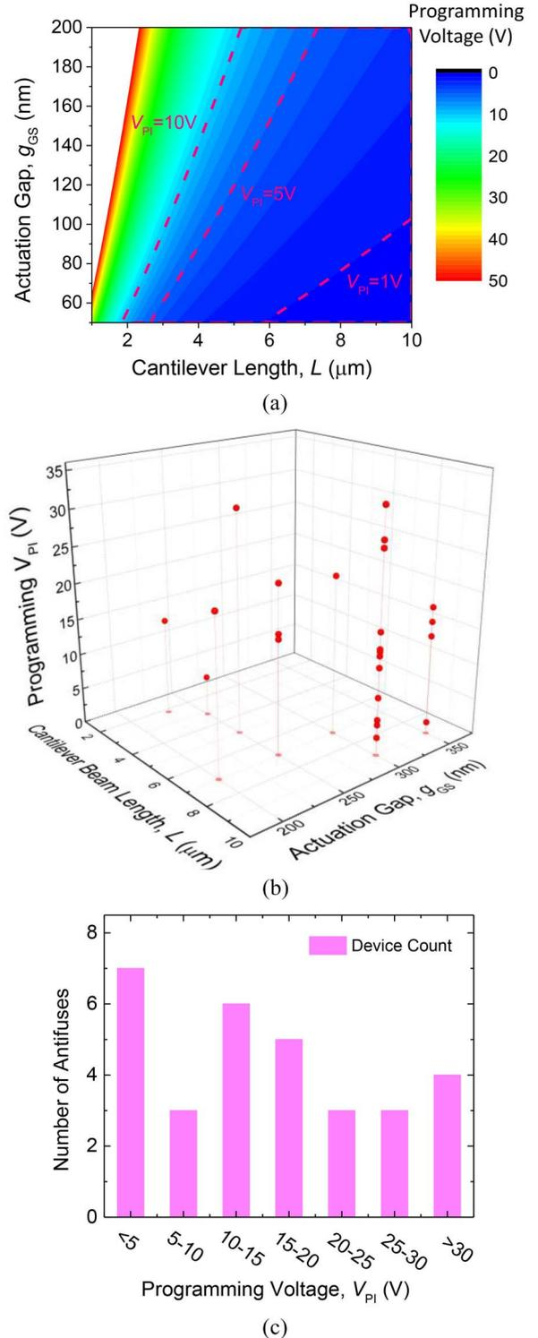
**FIGURE 8.** Programming voltage versus cantilever geometry. (a) Color map of calculated programming voltage versus actuation gap and cantilever length. (b) Measured programming voltage with designed actuation gap and cantilever length. (c) Histogram of measured programming voltage distribution across  $\sim 30$  NEMS antifuse devices.
