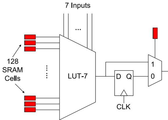
**FIGURE 13.** LUT-based C-cell logic blocks. The red blocks are the memory cells used to store information which can be replaced by NEMS OTP memory.
