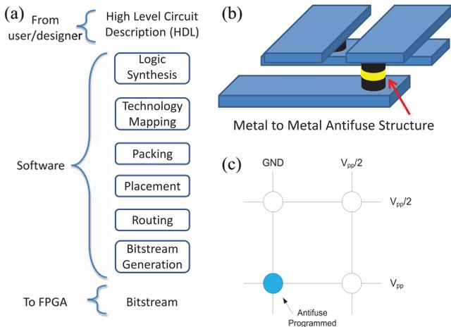
**FIGURE 10.** (a) Software flow of FPGA configuration. (b) Axcelerator family interconnect elements. (c) Programming scheme of applied voltages on Axcelerator family antifuses.
