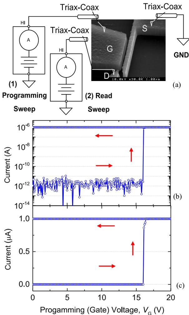
**FIGURE 14.** NEMS OTP memory cell characterization. (a) Programming scheme (1) and read scheme (2). Inset of (a) is an SEM image of a NEMS OTP memory cell. (b) and (c) Programming cycle through G with scheme (1), with current in logarithmic and linear scale, respectively.
