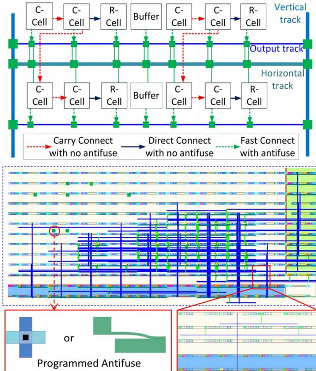
**FIGURE 12. Accelerator antifuse FPGA simulation architecture and layout of a mapped benchmark circuit. Top: FPGA architecture with logic modules (C-cell, R-cell, and buffers) and interconnections. Middle: layout of benchmark circuit after routing. Bottom: zoomed-in view of the programmed antifuses and circuit connections.**
