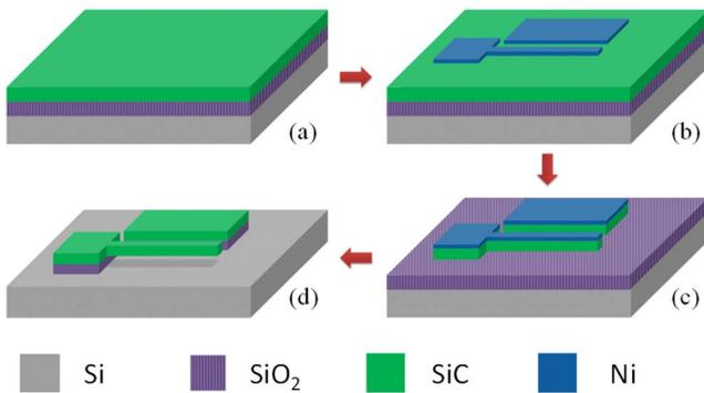
**FIGURE 3.** Nanofabrication of NEMS antifuse. (a) Poly-SiC deposited on 500 nm SiO<sub>2</sub> on a 4 in Si wafer. (b) 40 nm Ni layer after EBL and lift-off as the etching mask for SiC. (c) Reactive ion etching of SiC. (d) Ni removal and vapor HF etching of SiO<sub>2</sub> to suspend the nanocantilever beam.
