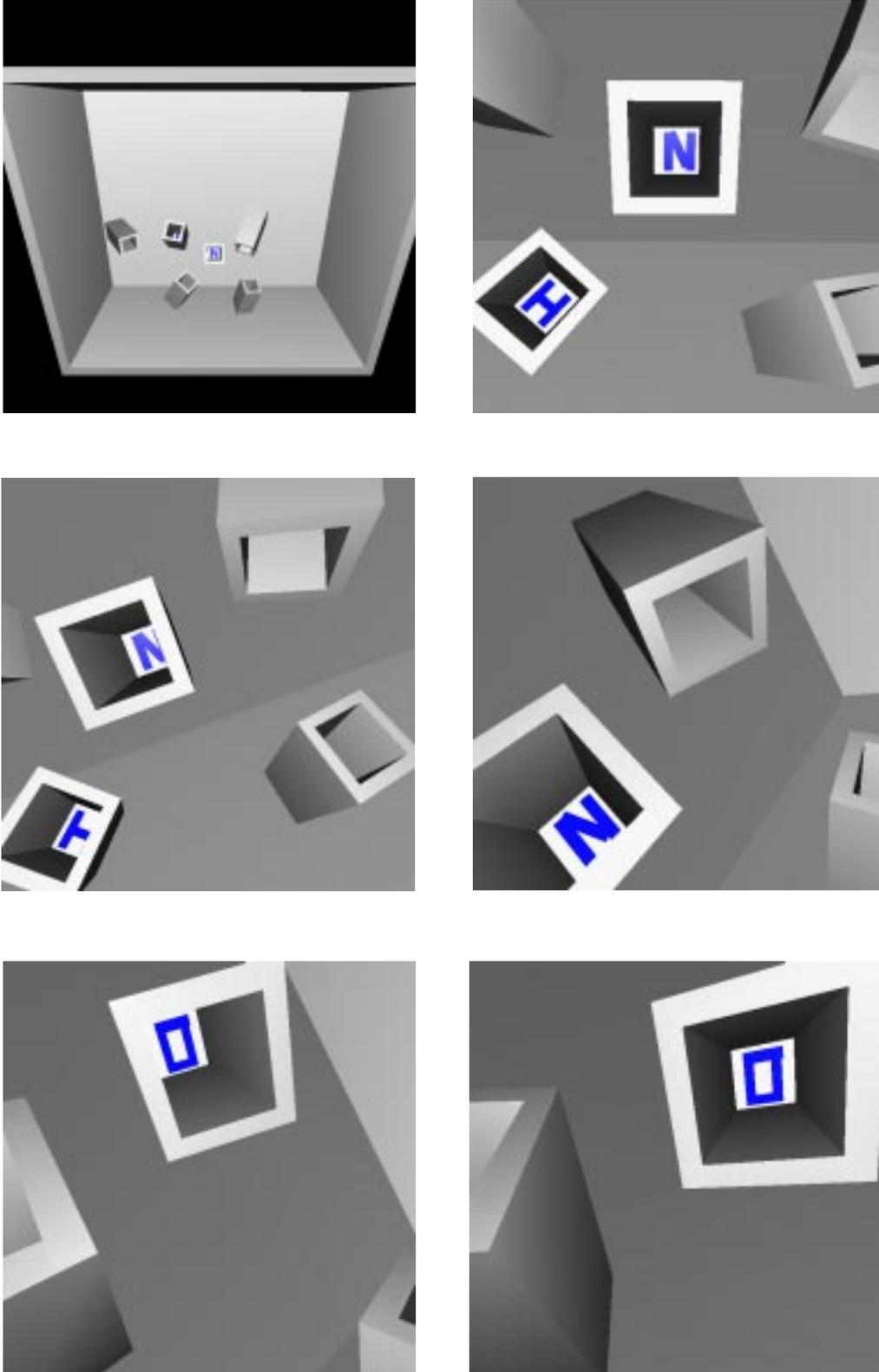
**Figure 3.** Angled laparoscope simulation. Upper left shows distant view of targets suspended at different positions and orientations. Remaining images show a sequence as the user smoothly changes the laparoscope position and orientation from view of target “N” to target “O”.
