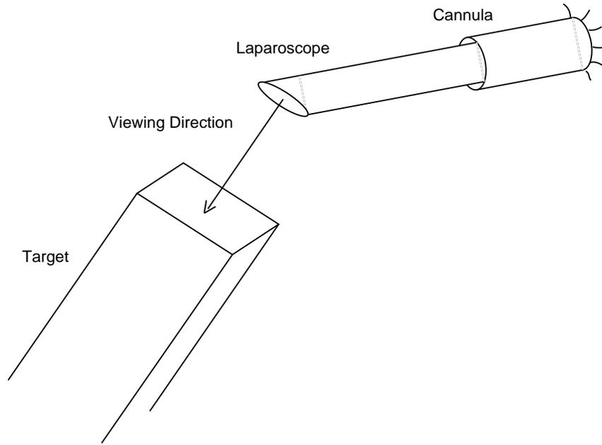
**Figure 2.** Angled laparoscope concept. The laparoscope passes through a cannula, which is constrained by the fulcrum at the abdominal wall. The objective lens is angled with respect to the laparoscope axis.
