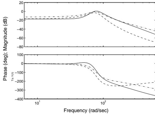
Figure 3. FREQUENCY DEPENDENCE OF (UNWEIGHTED) TRANSMITTED IMPEDANCE SENSITIVITY  $dZ_t/dZ_{env}$  AT  $Z_{env} = \hat{Z}_{env}$ . Solid line:KFF, dashed line: PERR, dash-dot line: P+FF.
