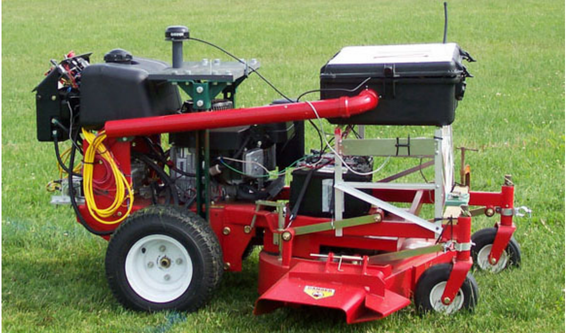
Figure 1.3: An autonomous lawnmower. Image courtesy Miami University and The Institute of Navigation.
