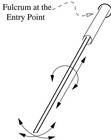
**Figure 1.** 4 DOF available in conventional laparoscopic instruments
