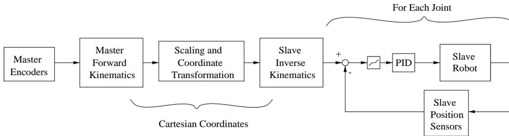
Figure 6. Current implementation of master-slave control
