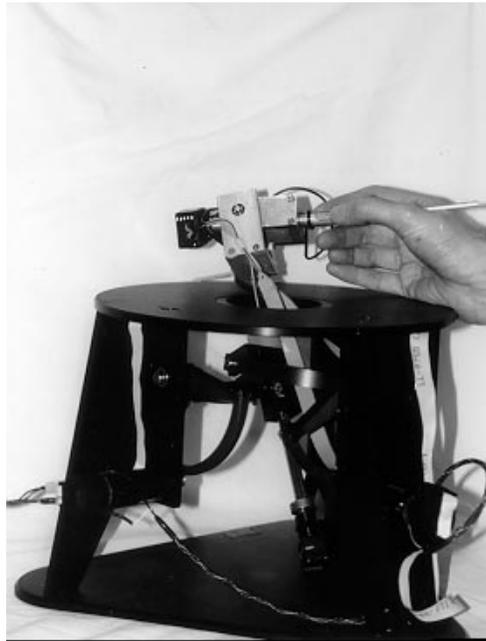
**Figure 4.** Master manipulator of the laparoscopic workstation
