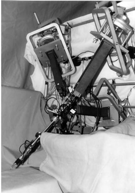
**Figure 2.** Slave manipulator of the Berkeley/Endorobotics/UCSF laparoscopic workstation
