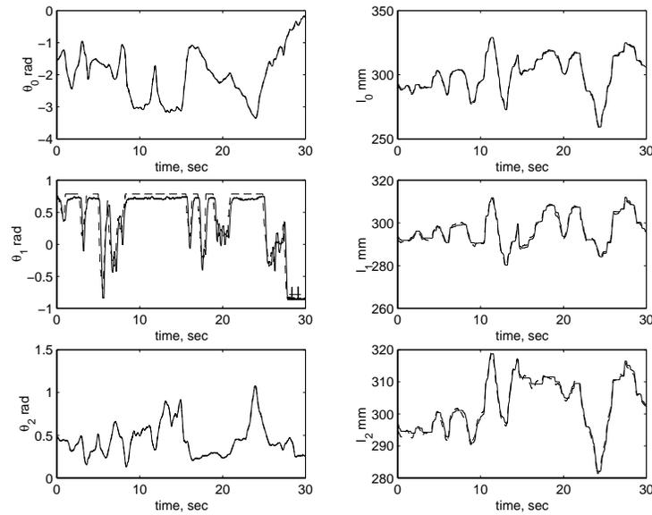
**Figure 7.** Master-slave tracking response: Dashed lines show the desired trajectory commanded by the master and the solid line show the actual trajectory of the slave.
