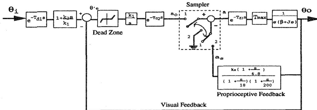
Fig. 3. Block diagram of sampled data control model for human hand tracking. Adapted from Navas and Stark, 1968.
